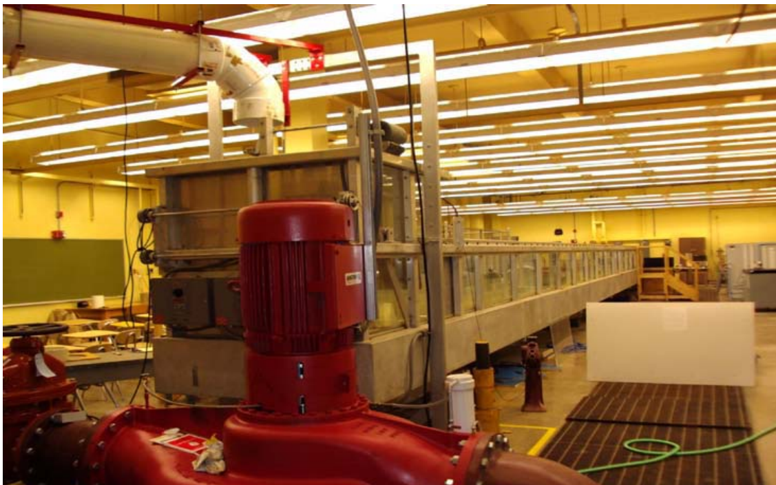
Fig: Laboratory set up of Flume and Pump
