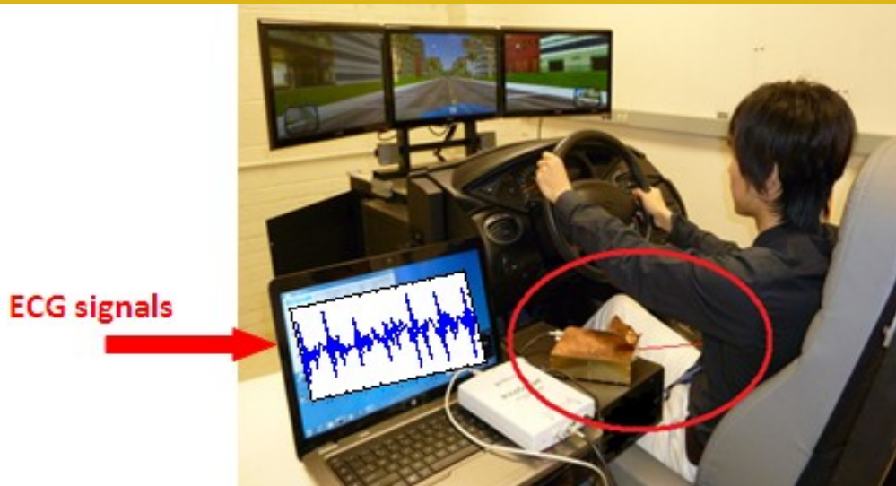
A non-contact ECG system monitors driver physiological signals at no interference to drivers.
