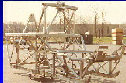
Current Alvin Frame Grade 2 Unalloyed titanium fabricated standard plate and pipe
