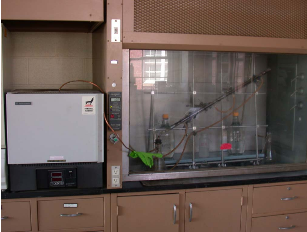
Fig. 6 – Laboratory Scale Yard Waste Carbonization Apparatus
