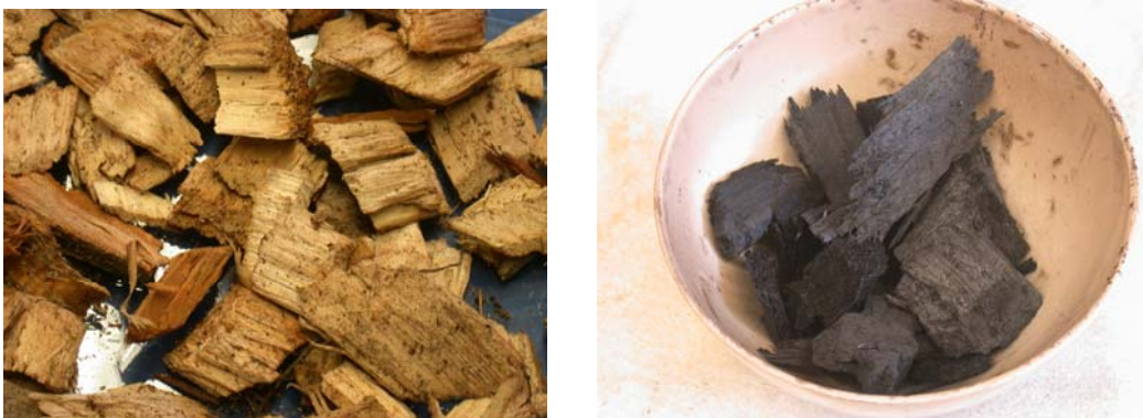
Fig. 7 - Hardwood chips before and after carbonization
