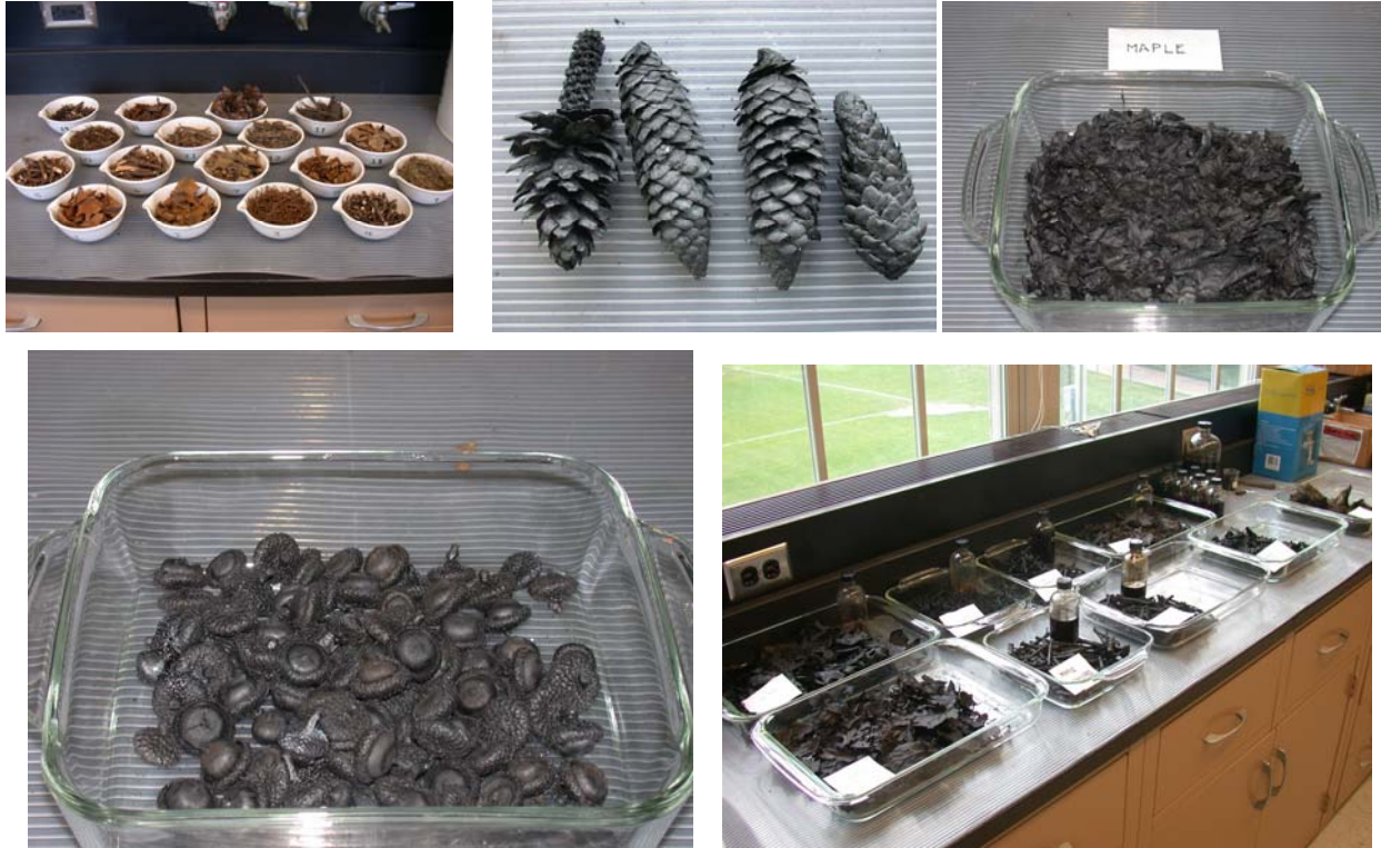
Fig. 8 Yard waste components before and after carbonization
