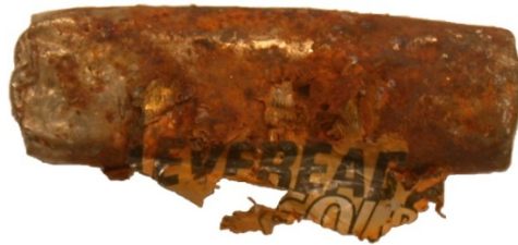
Figure 1: Battery Exhibiting Physical Damage Rating of 3 and Corrosion Condition rating of 2.
