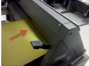
4. Slide the pinch rollers to the left and right edges of the vinyl sheet. Slide the rollers from the **back** of the cutter (not the front). The rollers must stay within the white markers above the rollers.
