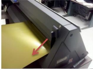
3. Insert the sheet from the back of the cutter, pulling it through to the front.
