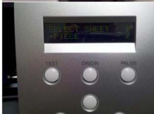
7. The cutter will slide the sheet backward & forward, measuring its dimensions.
