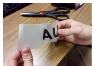
6. Stick the design on the desired surface, then carefully peel-off the transfer tape.
