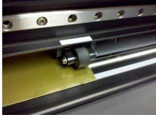
5. Tighten the platen by lifting the lever in the back-left of the cutter.
