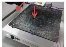
2. Unfasten spring clips around build plate edges, then **remove plate**.
