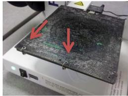
3. Reattach build plate. **Ensure all spring clips secure build plate**, otherwise plate may shift during printing.
