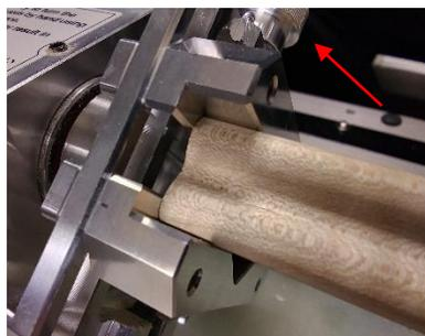
4. Slide tailstock so that its point touches material. Nudge material until tailstock point touches your mark.
