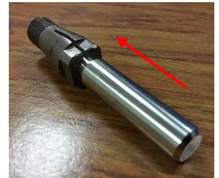
2. Insert collet & pin into machine's toolhead. Tighten with two black wrenches (push wrenches apart to tighten).
