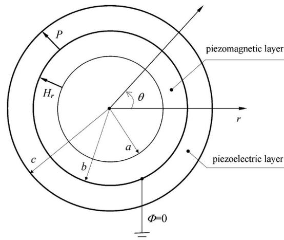
FIG. 1. Schematic of bilayer multiferroic cylindrical structure.
