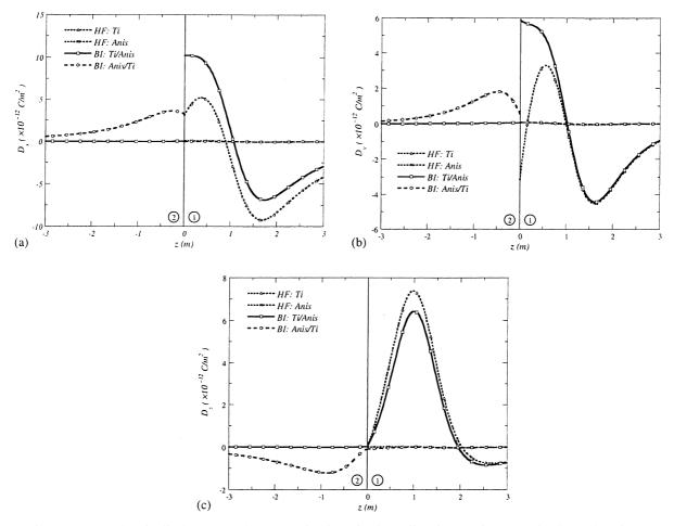
Fig. 4. Green's electric displacements due to a point force in the x-direction.  $D_x$  in (a),  $D_y$  in (b), and  $D_z$  in (c).
