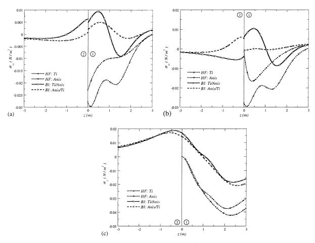
Fig. 6. Green's normal stresses due to a point force in the z-direction.  $\sigma_{xx}$  in (a),  $\sigma_{yy}$  in (b), and  $\sigma_{zz}$  in (c).
