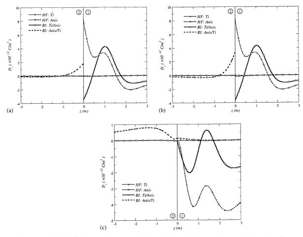
Fig. 7. Green's electric displacements due to a point force in the z-direction.  $D_x$  in (a),  $D_y$  in (b), and  $D_z$  in (c).
