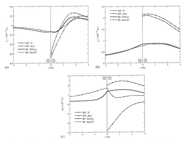
Fig. 5. Extended Green's displacements due to a point force in the z-direction.  $u_x$  in (a),  $u_z$  in (b), and  $\phi$  in (c).
