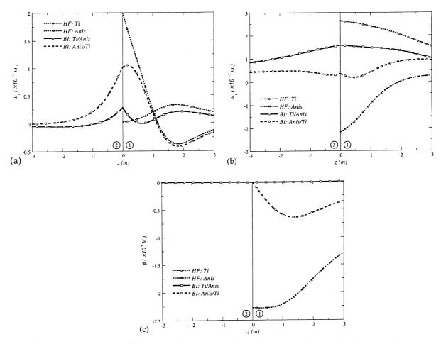
Fig. 8. Extended Green's displacements due to a negative point charge.  $u_x$  in (a),  $u_z$  in (b), and  $\phi$  in (c).
