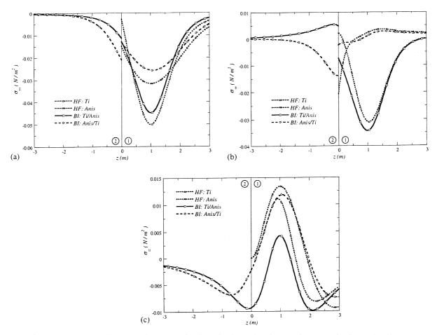
Fig. 3. Green's normal stresses due to a point force in the x-direction.  $\sigma_{xx}$  in (a),  $\sigma_{yy}$  in (b), and  $\sigma_{zz}$  in (c).
