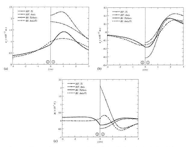
Fig. 2. Extended Green's displacements due to a point force in the x-direction.  $u_x$  in (a),  $u_z$  in (b), and  $\phi$  in (c).
