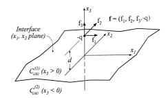
Fig. 1. An anisotropic piezoelectric bimaterial full space subjected to an extended concentrated force f applied at (0, 0, d) in material 1.
