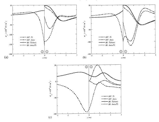
Fig. 9. Green's normal stresses due to a negative point charge.  $\sigma_{xx}$  in (a),  $\sigma_{yy}$  in (b), and  $\sigma_{zz}$  in (c).
