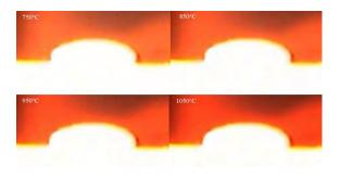
Wetting between metals and ceramics is of crucial importance to material joining and metal-matrix composite (MMC) production. Sessile drop method is one of the major techniques used on the investigation of metal-ceramic wetting. We investigate the contact angle of pure aluminum and aluminum-magnesium alloys on the surface of the polycrystalline alumina substrate in a broad temperature range (750 to 1100°C). Read more about Al/Alumina wetting and Al-Mg/Alumina wetting.
