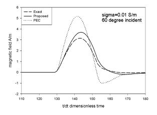
Fig. 4. Distribution of the magnetic field at the interface (2-D case).
