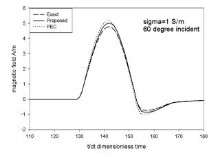
Fig. 5. Distribution of the magnetic field at the interface (2-D case).
