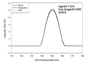
Fig. 3. Distribution of the magnetic field at the interface (1-D case).
