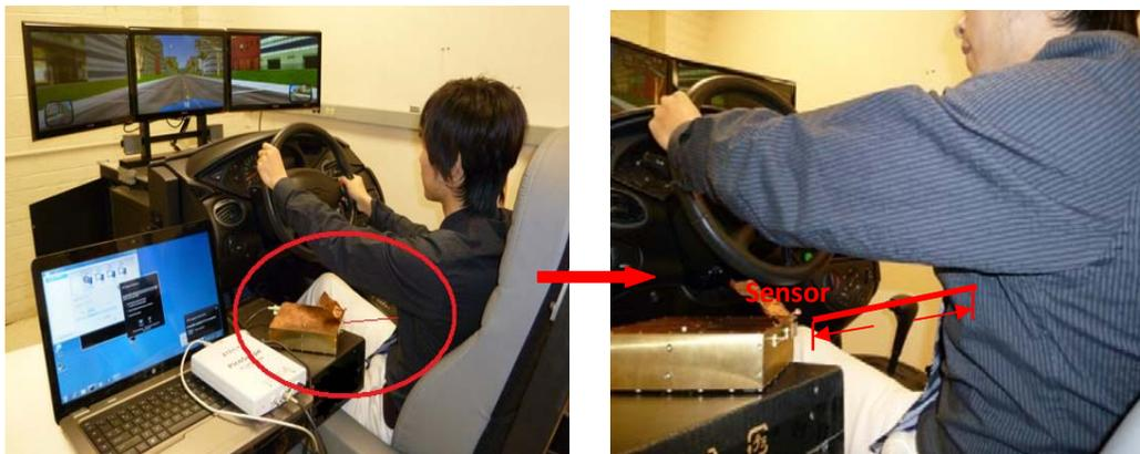
Figure 3 Detection system setup for ECG signal
