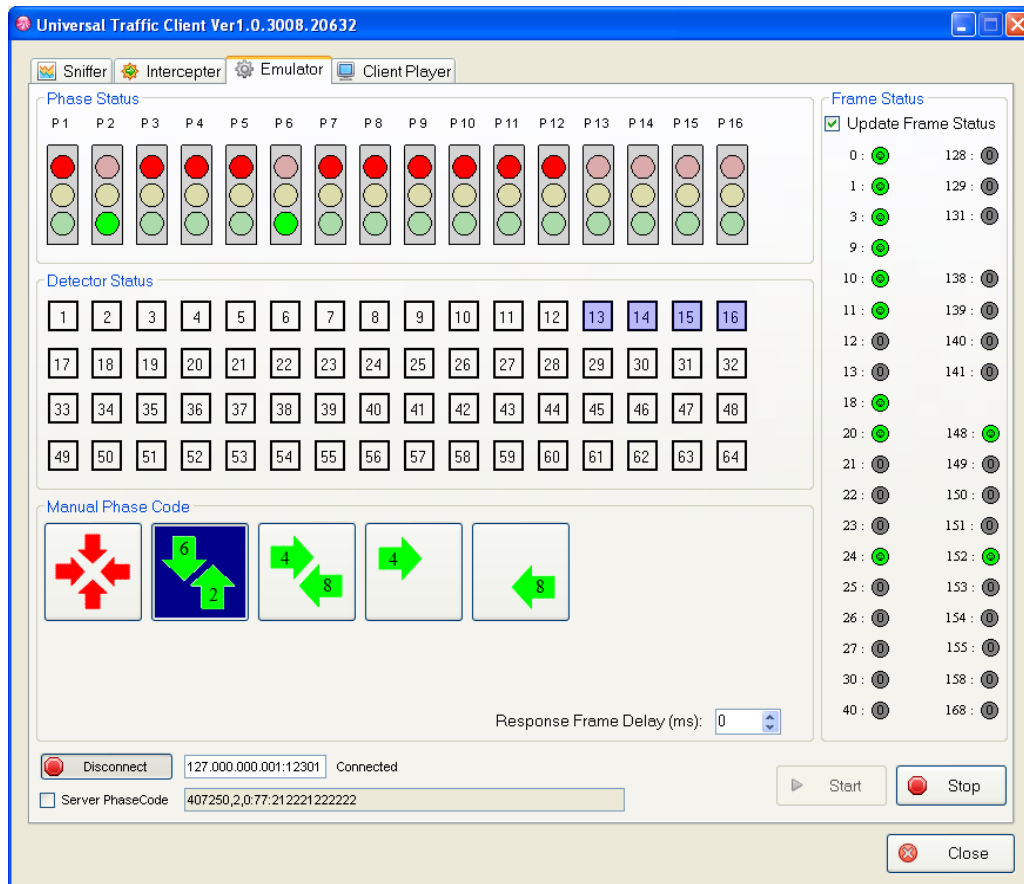
Figure 3.3 NEMA Standard Traffic Controller Emulator
