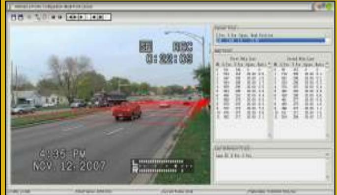
Fig. 1 Extract yellow onset speed & distance from stop line
