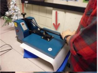
6. Watch the timer. When time's up, the heat press will beep. Lift the handle then remove your shirt.
