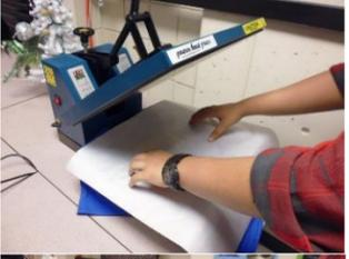
5. Close the heat press by firmly pulling down the handle until it locks into place.
