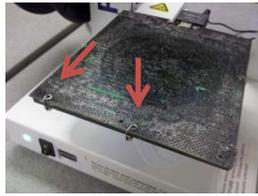
3. Reattach build plate. **Ensure all spring clips secure build plate**, otherwise plate may shift during printing.
