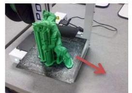
4. If your part has supports, wait for the part to cool completely to allow easy support removal.
