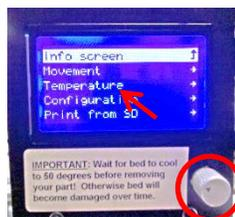
3. Highlight "Nozzle 1", press the knob, rotate the knob to "240", then press knob.
