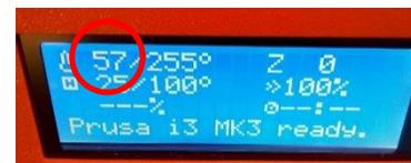
5. If you like the current filament choice, push the orange button again, then choose "Load to nozzle" from the menu. Then choose "Load filament X..." where "x" is the active spool tray from Step 1.
