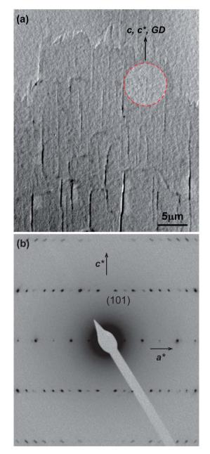
Fig. 6 (a) Bright-field TEM morphology of symTTF11 in the  $Col_K$  phase and (b) SAED pattern from the circled area of the bright-field TEM morphology in (a).
