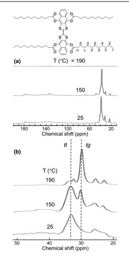
Fig. 8 Sets of solid-state  ${}^{13}$ C NMR spectra of symTTF11 during cooling between 190 °C and 25 °C with (a) CP/MAS/DD and (b) Bloch decay methods.
