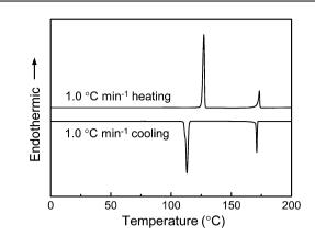
Fig. 2 A set of DSC cooling and subsequent heating thermal diagrams of symTTF11 at 1.0 °C min<sup>-1</sup>.
