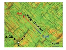
Fig. 4 POM image of the oriented symTTF11 crystal grown on the temperature gradient surface between 200 °C and 25 °C. Here, GD means the growth direction and xyz Cartesian coordinate represents the symTTF11 sample geometry in a real space.
